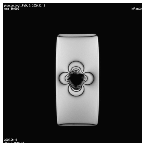
Fig. 5. Typical susceptibility artifacts of a balanced steady-state free precession (bSSFP) sequence showing T_2/T_1 -contrast. ( TRUFI -sequence: TE = 2.15 \text{ ms} , TR = 4.3 \text{ ms} ; \alpha = 74^\circ .) For materials and experimental setup see Fig. 4.
